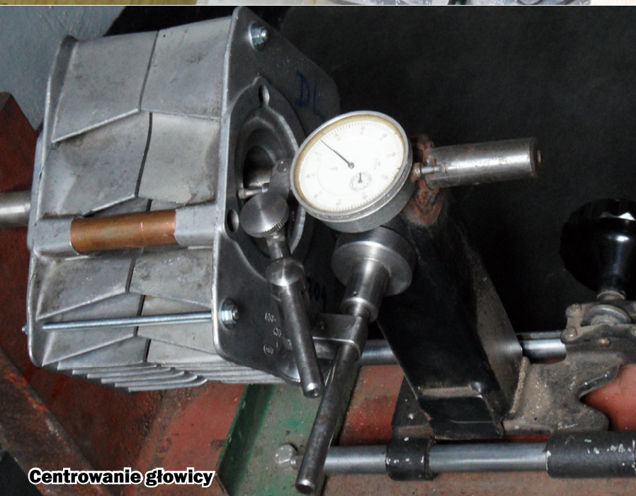
Cylindry górne na stole frezarki
